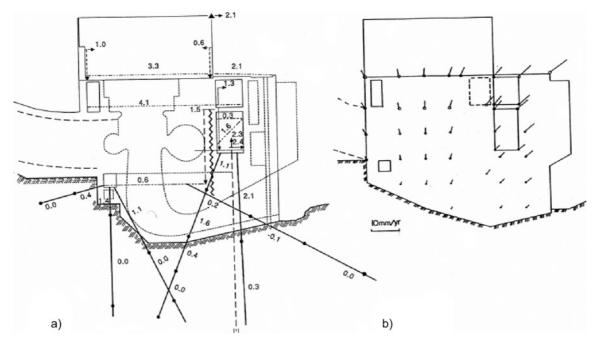
Figure 1: Application of the Generalized Method of geometrical analysis (after Chrzanowski 1993): a) observed rates of deformation (mm/y), b) derived displacement field.
