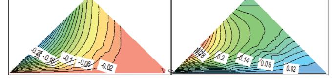
Figure 2: Predicted displacements [m] after filling the reservoir. a) vertical displacements, b) horizontal displacements.
